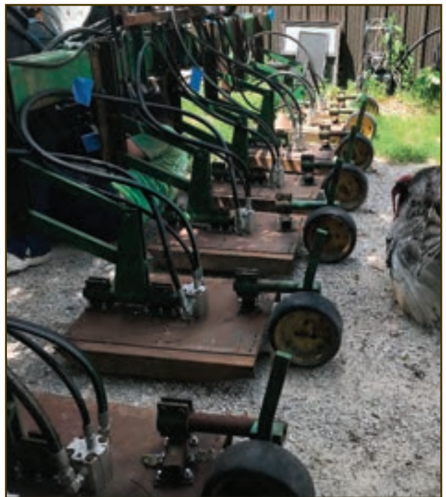
Figures 2-3. Mowers in production at the University of Missouri that were converted from old cultivators through collaboration with a stakeholder who received a SARE farmer-rancher grant.
