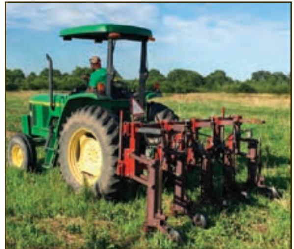
Figure 1. Photo of between row mower designed and built at the University of Missouri.
